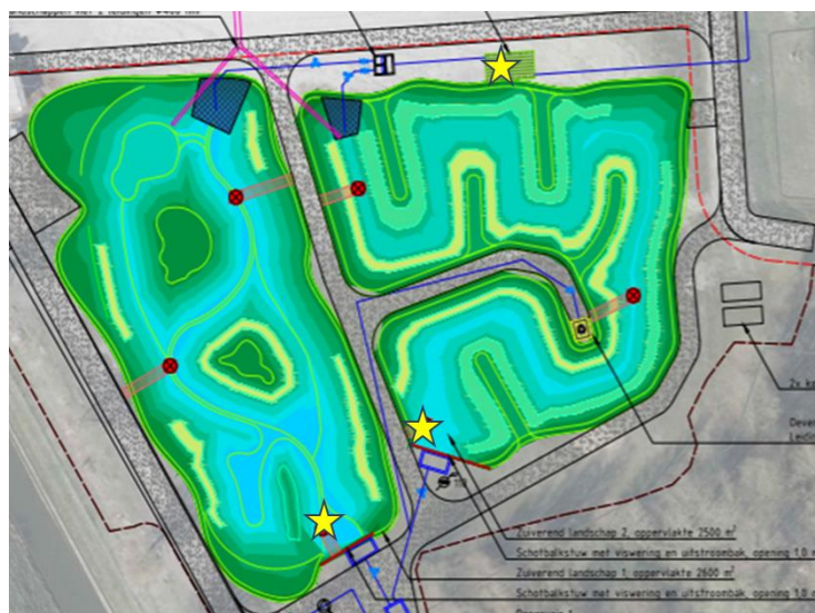
Figure 5. Locations of online monitoring systems. Yellow stars indicate the positions of the sensors, with one sensor located in the mussel zone and one at the outlets of each landscape.
