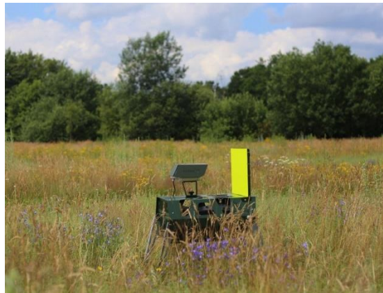
Figure 7. DIOPSIS camera system used to monitor flying insects. AI software processes the images to identify species.
